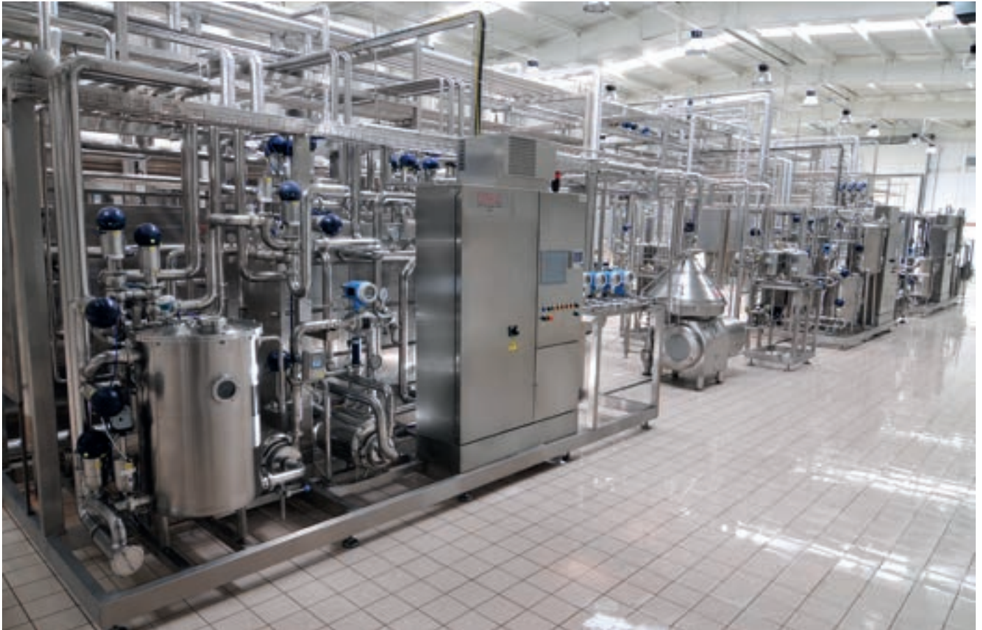
Complete line of milk pasteurisation with in-line automatic standardization system for milk/cream
