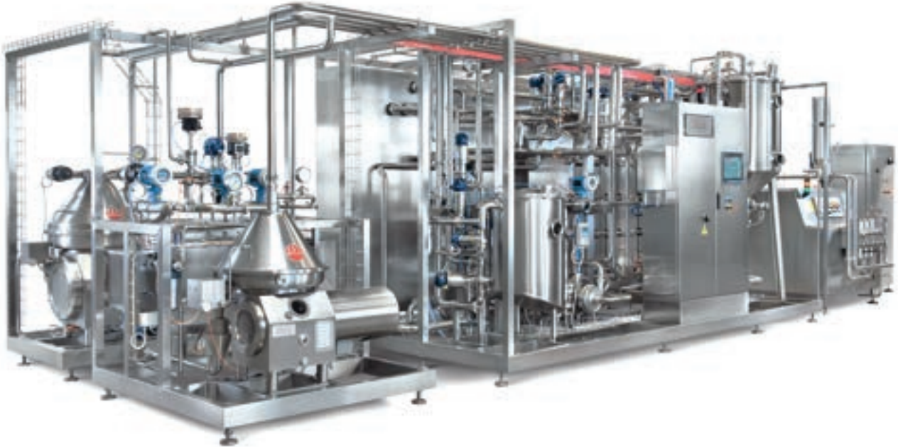
Complete line for 10,000 l/h of ESL milk with bactofuge, milk/cream separator, automatic in-line standardizer, deaerator/degaser and homogenizer
