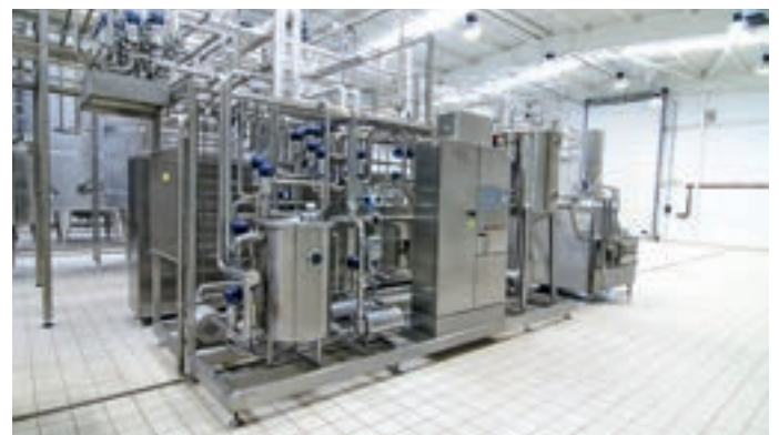
Complete line of milk pasteurisation with in-line automatic standardization system for milk/cream
